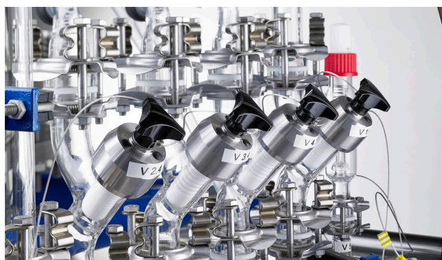
Valve arrangement of the vacuum connection
