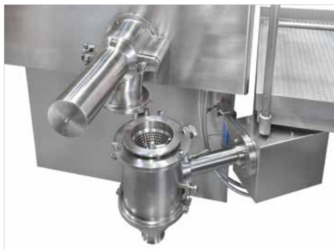
MGT with integrated wet sieve
