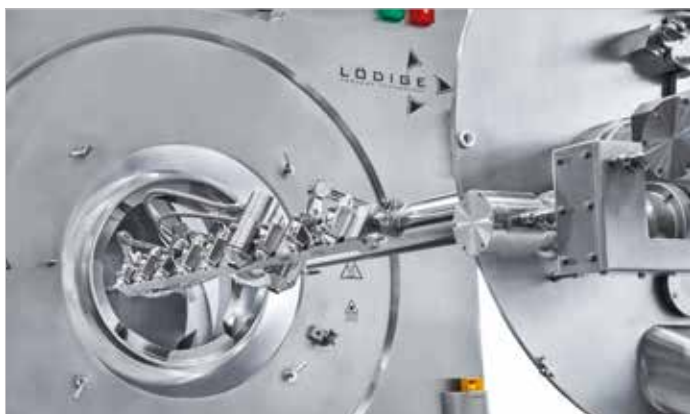
Lödige Coater type LC 150 with spray arm in run-out position
