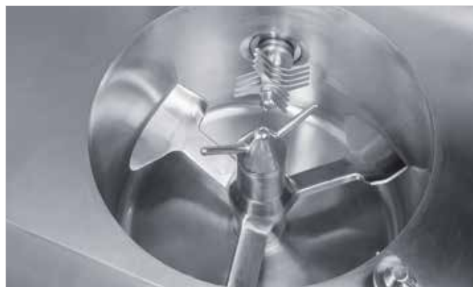
Three-arm mixing element and chopper
