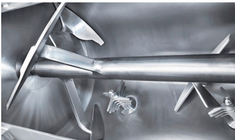
Fully welded mixing elements without any gaps or dirt traps (Hygienic Design)
