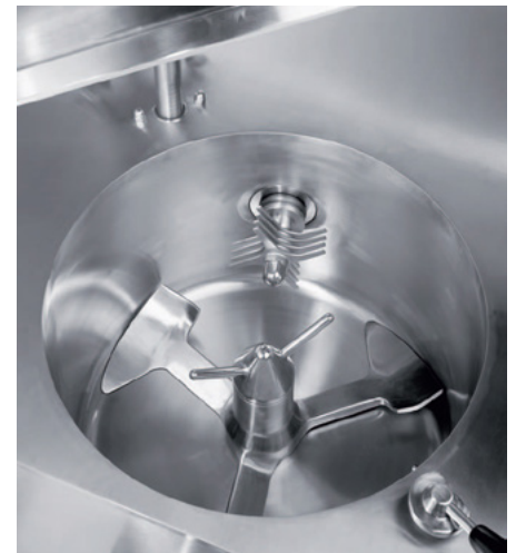
Mixing tool which can be raised up
