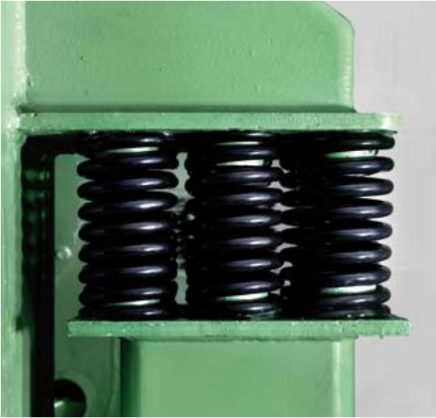
Swinging body supported on steel springs
